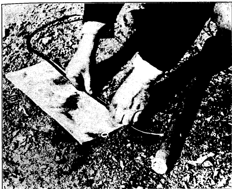
FIGURE 84. Determination of the Velocity of Detonation of Dynamite by the Dautriche Method. (Courtesy Hercules Powder Company.) Compare Figure 9, page 17.
