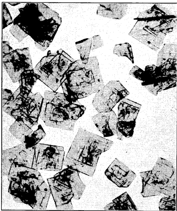
FIGURE 103. Diazodinitrophenol Crystals (90 \times ).
