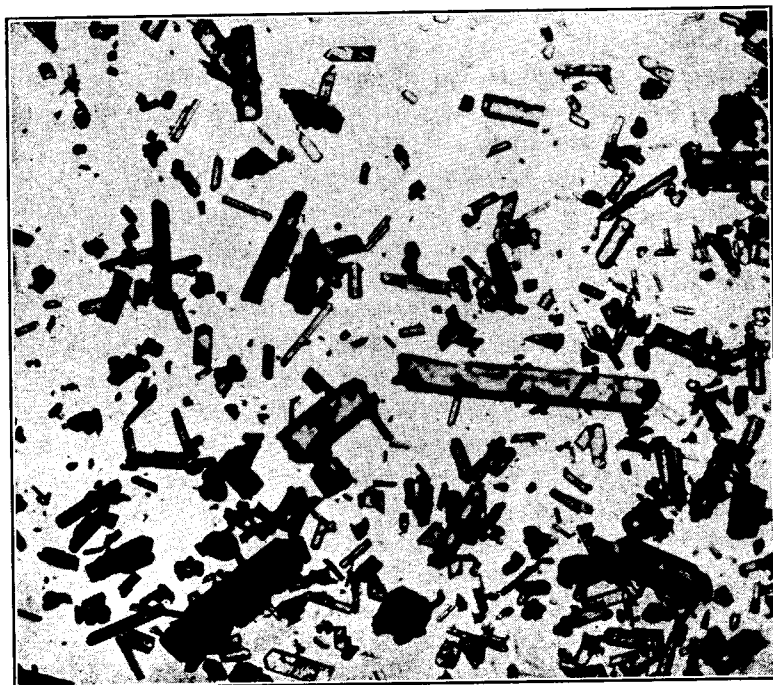
FIGURE 49. Commercial Sample of Ammonium Picrate (25×).
