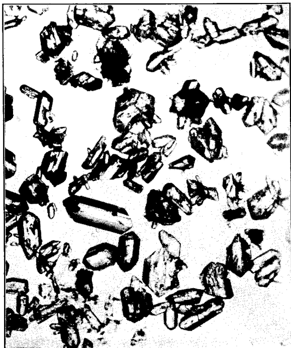
FIGURE 102. Lead Styphnate Crystals (90×).
