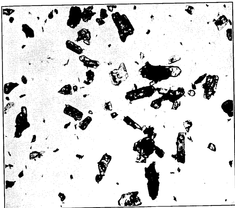
FIGURE 47. Commercial Sample of Purified TNT (25 \times ).
