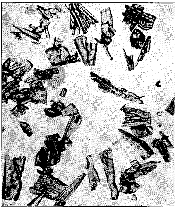
FIGURE 104. Tetracene Crystals (150 \times ).
