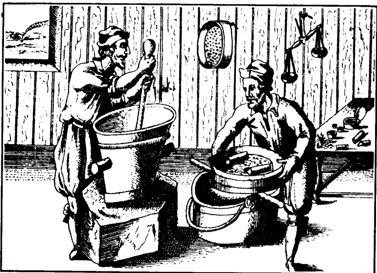
FIGURE 18. Gunpowder Manufacture, Lorraine, 1630. After the materials had been intimately ground together in the mortar, the mixture was moistened with water, or with a solution of camphor in brandy, or with other material, and formed into grains by rubbing through a sieve.
