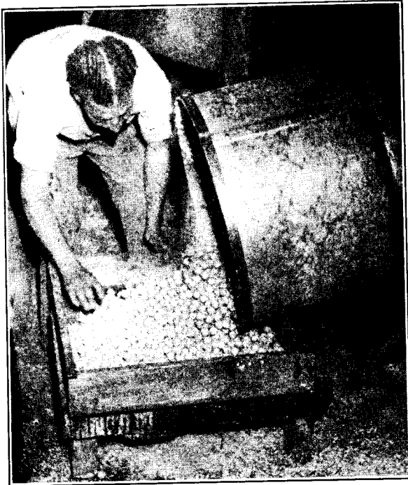
FIGURE 35. Manufacture of Globe Torpedoes. Removing the moist spheres from the tumbling barrel. (Courtesy National Fireworks Company and the Boston Globe .)
