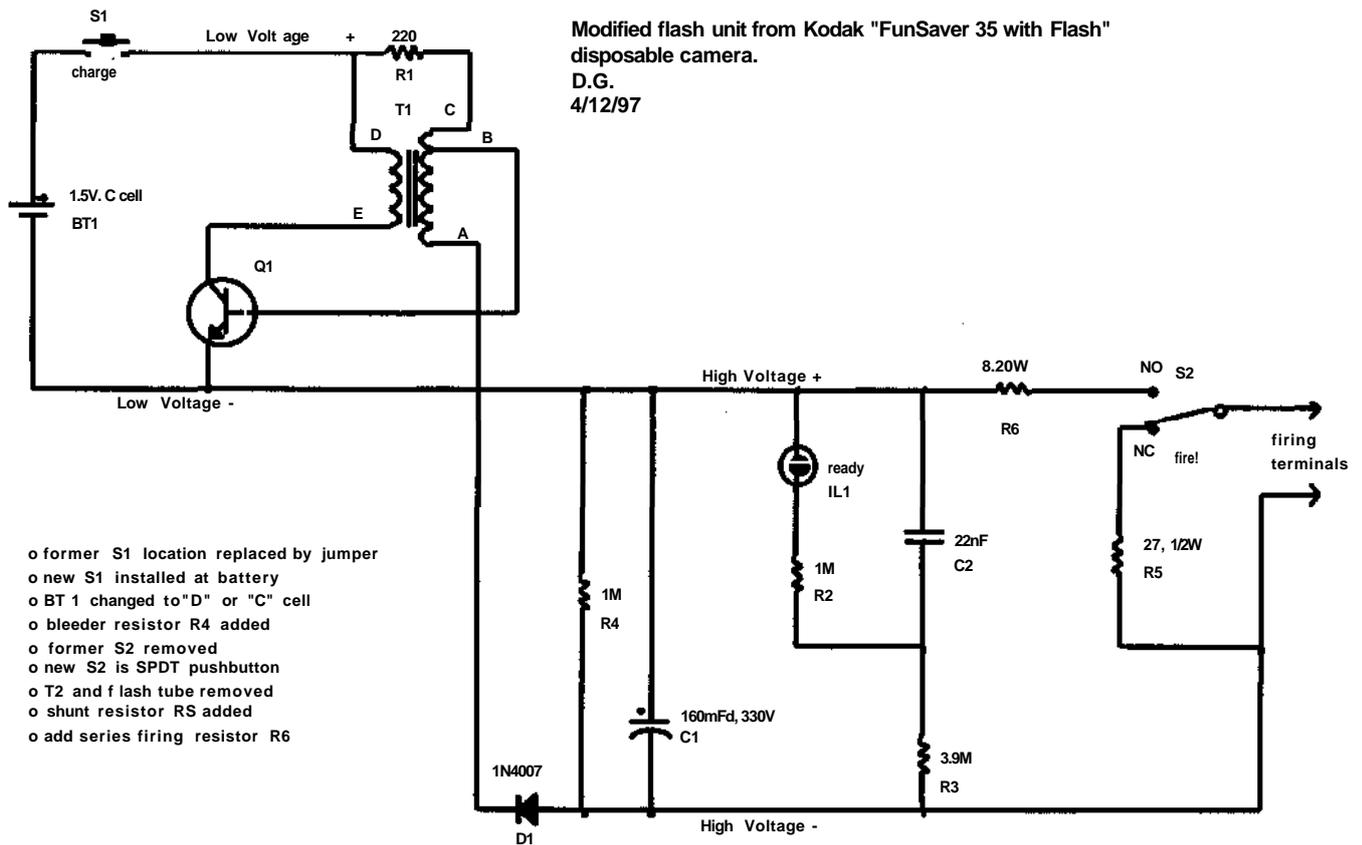
Figure 4 - Mechanical switch variation of CD firing box.
