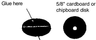
Disk, brad, and wire support assembly. Place dab of hot melt over the hole in the middle to secure the brad.
