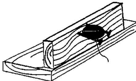
A simple jig for holding the disk assemblies. This saves on burned fingers when applying the hot melt glue used to secure the brad and wire to the cardboard disk.
