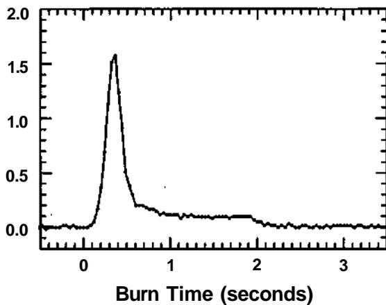
Figure 4. Typical thrust profile of a Sky Bloom rocket.
