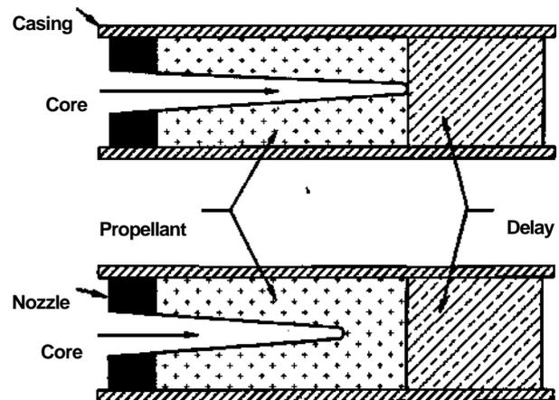
Figure 3. Rocket motors with varying core length.
