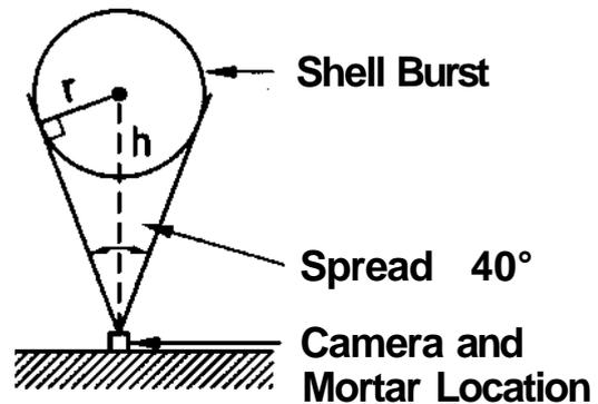
Figure 2. Geometry of a typical hard breaking spherical shell
