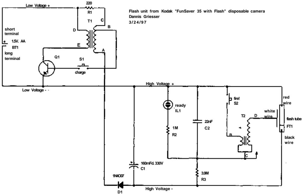
Figure 2 - Flash circuit schematic diagram
