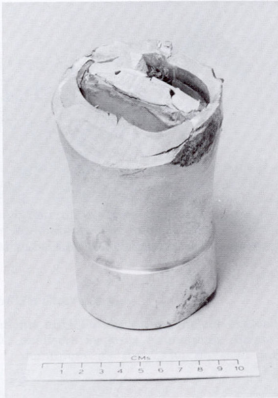
FIG. 8.2 Undersea cable cut for a guillotine cutter
