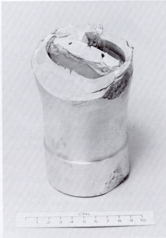
FIG. 8.2 Undersea cable cut for a guillotine cutter
