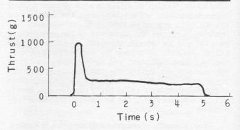
Figure 3. Thrust-time curve for a hollowed burning surface.
