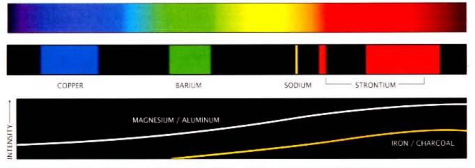
FIREWORKS GLOW by incandescent, atomic, and molecular emission. The color depends on where the emission falls on the visible spectrum (top). Atoms and molecules become excited at the high temperatures in a pyrotechnic flame and release their excess energy as light. Atomic sodium is an intense yellow-orange emitter. Fragile compounds containing
