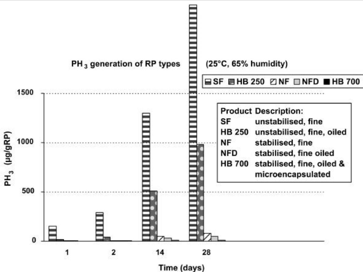
Figure 6. PH<sub>3</sub> generation of red phosphorus types.
