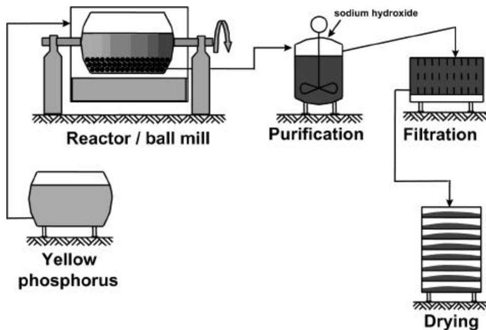
*Figure 1. Production of red phosphorus.*
